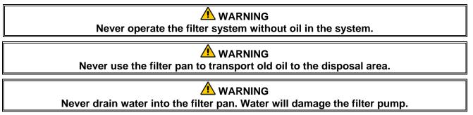
There are no periodic preventive maintenance checks and services required for your FootPrint Pro Filtration System other than daily cleaning of the filter pan with a solution of hot water and McDonald's All Purpose Concentrate.
