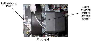
The air/gas mixture is properly adjusted when the burner manifold pressure is in accordance with the applicable table on page 2-4 and the burners display a bright orange-red glow. If a blue flame is observed, or if there are dark spots on a burner face, the air/gas mixture requires adjustment.
