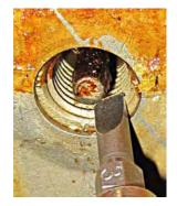
3. Note the temperature on the thermometer or pyrometer. Actual temperature and pyrometer readings should be within  $\pm 5^{\circ}F(3^{\circ}C)$  of each other. If not, contact a Factory Authorized Servicer for assistance.
