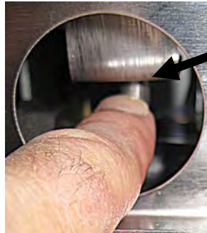
Filter Pump Reset Switch
