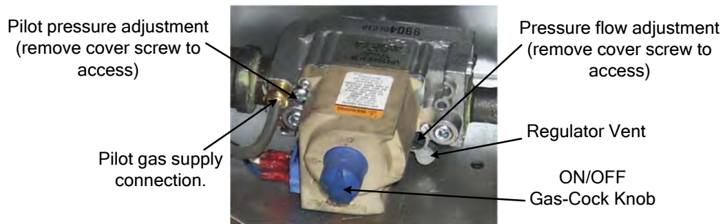
Typical non-CE gas valve for electronic-ignition equipped fryers.
