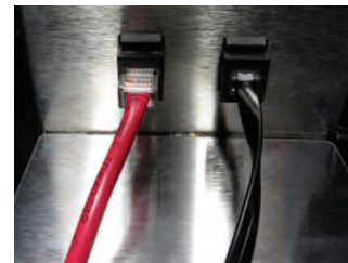
Figure 2: The translator connects to the primary holding cabinet with RJ12 cable (right). The secondary cabinet, if present, is connected with CAT 5 cable (left). The primary cabinet must be larger or equal in size to the secondary cabinet.
