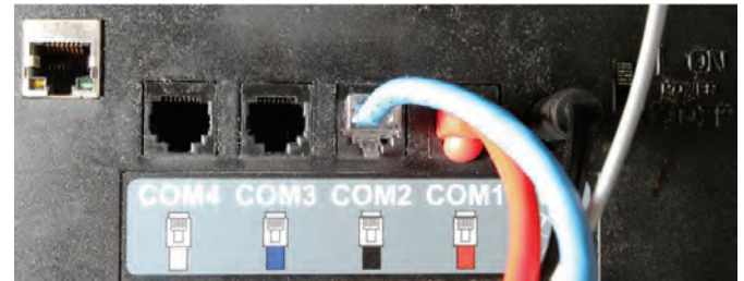
Figure 1: COM ports on the back of the Kitchen Minder are connected to Merco Translators, which are in turn connected to a Merco holding cabinet.
