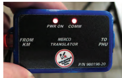
Figure 3: The PWR LED is illuminated when the network is active. The COMM LED should only show a weak intermittent blink, which indicates successful network activity. A bright flashing COMM LED is indicative of a network communication issue, often associated with cables. The translator box above is unplugged from the holding cabinet.
