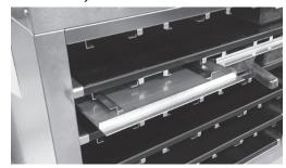
7. Clean the trays, RFID bands, RFID collars, RFID carriers, lids, false bottoms and tray seals in a dishwasher or with warm soapy water.
