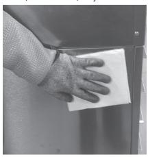
10. Wipe the interior with a damp cloth; clean from the front and the back to reach all surfaces. Pay attention to the ledges that support tray seals. If an excessive amount of food particles/grease has collected, hot sudsy water (non-abrasive) may be used.
