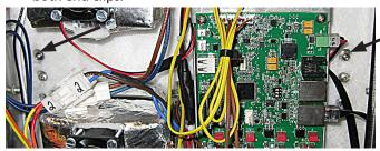
4. Remove the the bracket holding the antenna by removing the nuts on the back.
