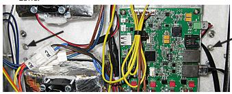
6. Thermocouple connections are at the top of the IO board. Mark plugs for reassembly. Pay close attention to their placement. From both sides of the cabinet unplug
