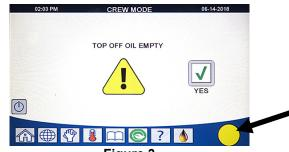
Figure 3 Yellow indicator that oil reservoir is empty.
