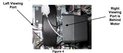
The air/gas mixture is properly adjusted when the burner manifold pressure is in accordance with the applicable table on page 2-4 and the burners display a bright orange-red glow. If a blue flame is observed, or if there are dark spots on a burner face, the air/gas mixture requires adjustment.
