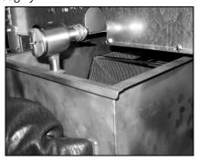
Inspect the filter pan connection fitting to ensure that both O-rings are in good condition (See Figure 2). Ensure the pre-filter screen is installed, clean and tight.
