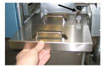
**Figure 4**: Place the lid on the pan and slide the oil pickup tube into the female suction receptacle.
