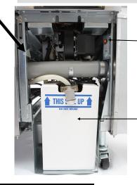
D: Top off reset button: Press and hold after replacing the oil/shortening until yellow indicator goes out.
