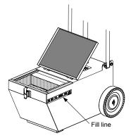
4. Carefully withdraw the unit far enough to allow the cover to be closed. Latch the cover in the closed postion. Using the handle, carefully tip the unit back slightly for ease of handling and roll the unit to the disposal site.
