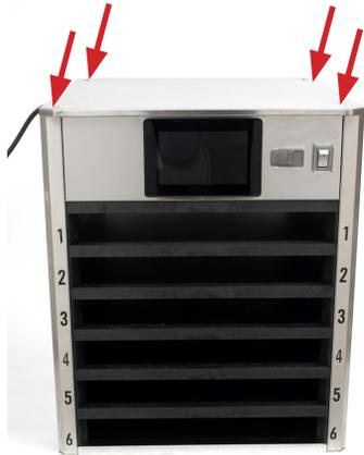
3. Remove both sides, by removing the two (2) Phillips head screws at the bottom of the each side panel and sliding up and away from the cabinet.
