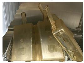
5. Wipe the interior shelf with a damp cloth. If, however, an excessive amount of food particles/grease has collected, hot sudsy water (non-abrasive) may be used on the cloth.
