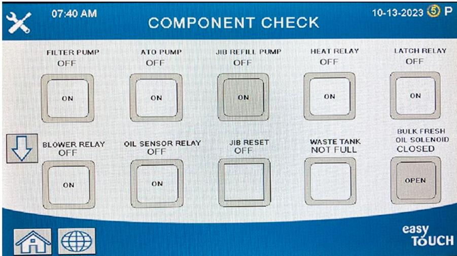
Pressing the home button to exit the function will display driving valves to ensure all valves return to home state. Once completed the controller will display FILL VAT FROM DRAIN PAN? YES NO. Press YES to ensure that any oil in the filter pan is returned to the vat.
