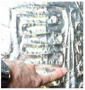
The heater thermocouple (brown wire) is under the same tape as the heater. Failed thermocouples require a heater replacement.
