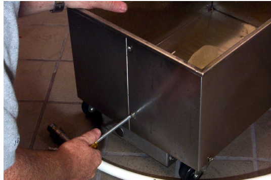
Remove screws securing outer panels.
