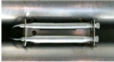
Typical high-limit/sensor probe locations and mounting hardware.
