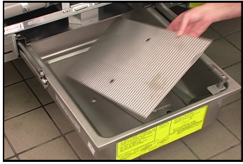
Place the inner screen in first (above) and then the filter paper (below).
