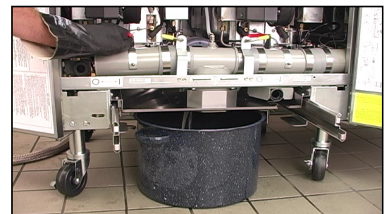
Drain slowly into a metal stockpot. Do not drain into the filter system or an SDU.
