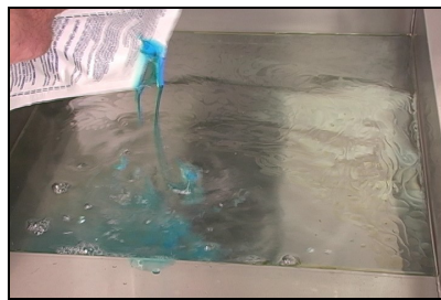
Add cleaning solution to water in the frypot.
