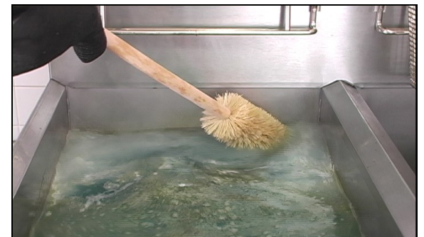
Scrub stubborn stains with a brush as the cleaning solution soaks in the frypot.
