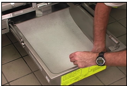
Place the inner screen in first (above) and then the filter paper (below).
