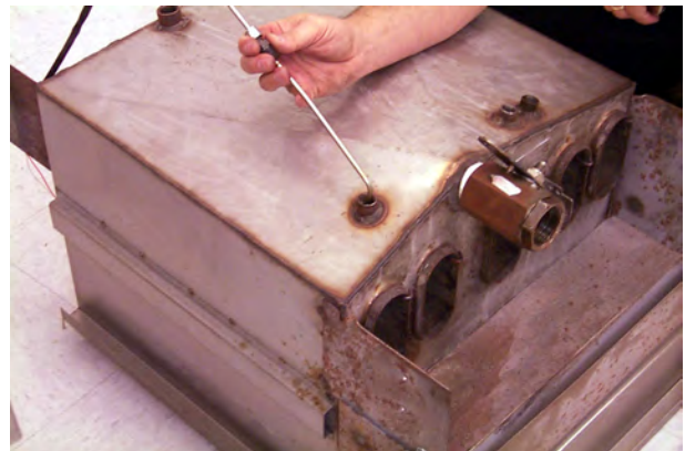
After removing the probe mounting hardware, the temperature probe can be removed through the bottom of the frypot. Retain the mounting hardware for reassembly.
