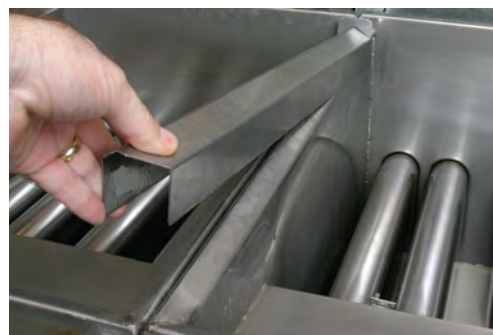
Removing the joiner strip.
