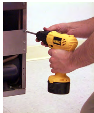
Removing gas manifold shield.
