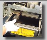
• Ensure the filter pan is in place and all components removed & tap Yes.
