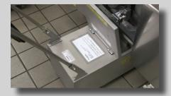
• Place Cleaning Disposal Unit capable of holding four gallons under fryer at prompt and tap Yes once in place.
