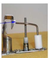
After the electrode is positioned and properly adjusted, ensure the flame completely engulfs the flame sensor at all times during operation. Check the pilot flame with all frypots heating to ensure
