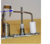
The electrode position in relation to the pilot hood deflector is crucial to accurate ignition. If the electrode is out of adjustment, the spark current will seek an alternate path to the flame-sense rod, causing ignition
