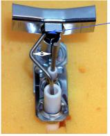
The electrode tip is properly positioned just under the pilot hood deflector corner. (Note orientation of electrode in relation to deflector corner.)
