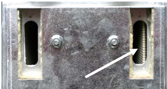
Figure 1: The burner ceramic should not be readily visible when looking straight into the igniter port. The burner in this misaligned frypot (see arrow) extends into the path of the igniter.
