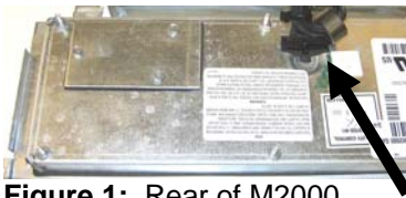
Figure 1: Rear of M2000 SMT computer. Unplug the 20-pin plug.
