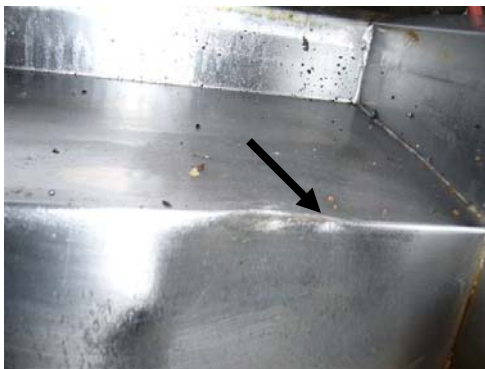
Figure 2: Banging a basket to dislodge oil leads to dents like those shown above. Overtime, hairline cracks can develop and in extreme cases (shown at right) the frypot can be punctured. Such damage is not covered by warranty.
