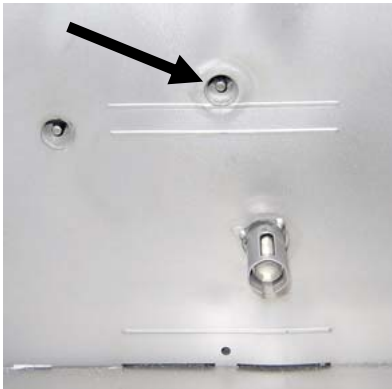
Figure 6 Lower oil level beneath this sensor on electrics.
