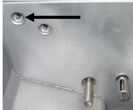
Figure 7 Lower oil level beneath this sensor on gas.
