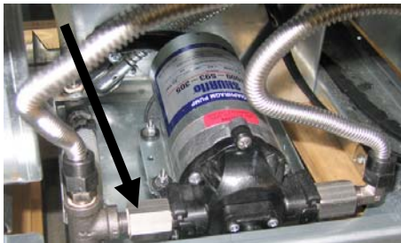
Figure 1 Release quick disconnect on inlet side.
