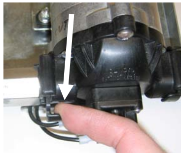
Figure 2 Release quick disconnect by pulling keyhole release.
