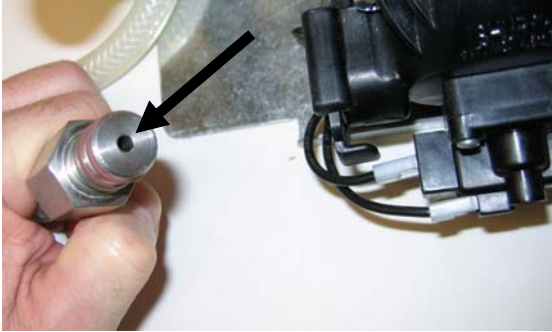
Figure 4 Blow compressed air through inlet side to JIB.
