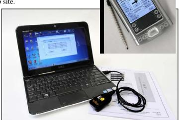
A minicomputer, special UHC-P software and an infra red communication device are replacing the Palm Pilot (inset above right) as a means of programming the UHC-P cabinet.
