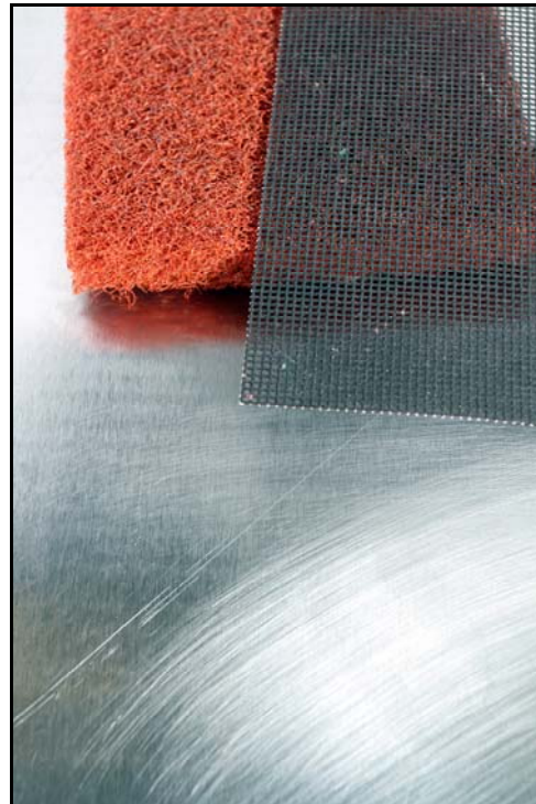
Damage caused with just a small amount of scrubbing.
