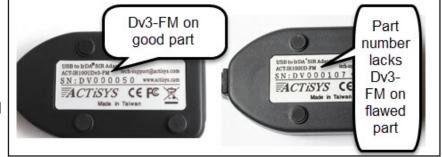
The flawed dongle is shown above (right). It is identifiable by the serial number range and the absence of a -3 in the part number. The good part, with the -3 in the part number is shown on the left.
