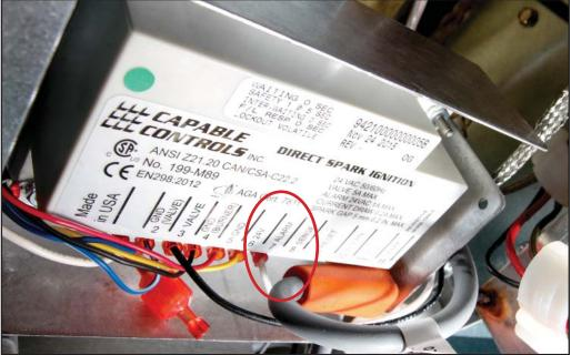
The alarm wire (in circle) should be removed on left-side Capable Controls spark modules for full vat H50, H55, LOV, GL30, OCF or FilterQuick fryers with two spark modules. The left-side alarm circuit is unnecessary on single vats with two Capable Controls spark modules. Timing issues between the right and left modules in the alarm circuit can cause nuisance alarms.
