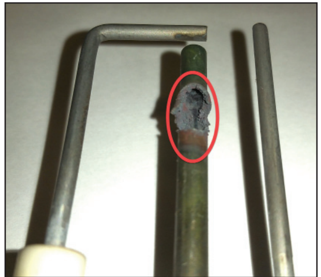
Figure 1: Igniter enrichment tube damaged by high-pressure or high caloric value propane-butane gas mix.
