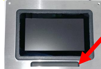
Figure 2 Front of Replacement Controller for Older Style Controllers with Cooling Louver
