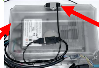
Figure 3 Rear of Replacement Controller for Older Style Controllers with housing and fan.
