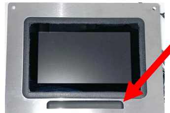
Figure 4 Front of Replacement Controller for Older Style Controllers with Cooling Louver
