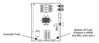
3. Replace the component box cover, being sure to reconnect the ground wire with the upper left screw.
