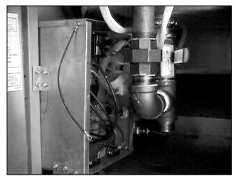
5. Replace the component box cover, being sure to reconnect the ground wire. Replace any drain plumbing components that were removed and reconnect the cooker to the electrical power supply.
