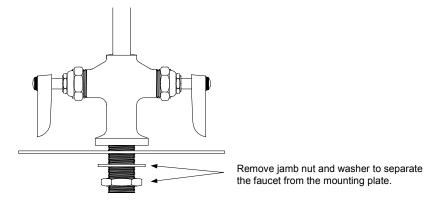
8. Assemble the replacement faucet to the mounting bracket and complete the procedure by reversing Steps 1-6.
