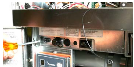
Figure 2: Remove access panel under computer.
